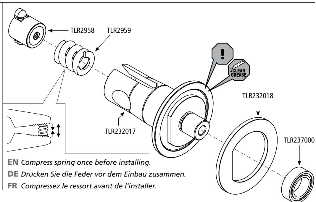
**EN** Compress spring once before installing.
